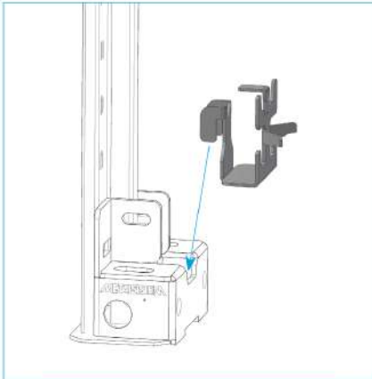
1 - Bracket slots over reinforced base plate
